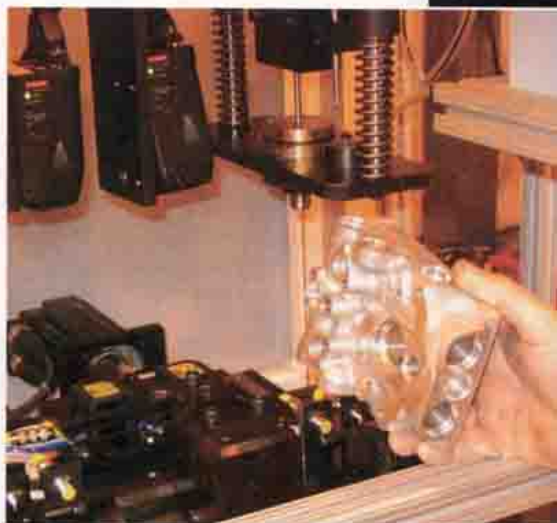
Delphi Automotive Systems reads dot-peen data matrix codes on top of braking system part (above). Microscan Quadrus EZ smart camera (right) shows the 2D code on screen, without exterior lighting.
