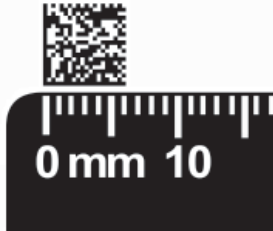
Figure 2: 50 characters encoded in a small symbol. Graphic is to scale but not actual size.
